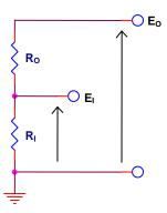
Figure 16. Non-Inverting Amplifier Analyzed as a Voltage Divider
