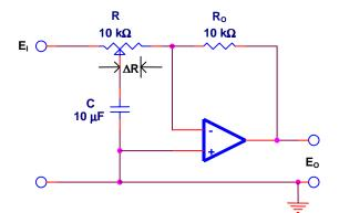
Non-integrating type. Constant inverting unity gain. Maximum lag for R centered for  $\Delta = \frac{1}{2}$  where  $0 \le \Delta \le 1$  is the log setting.
