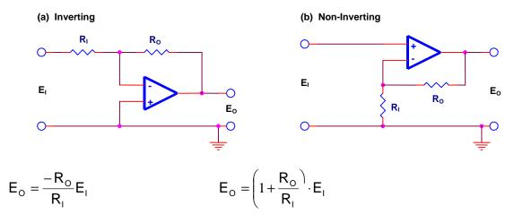
Figure 11. Basic Amplifier Circuits
