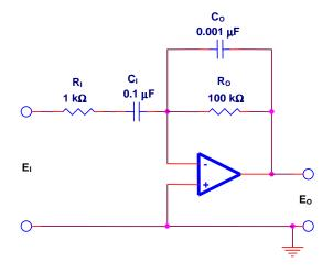
$R_1C_1 = R_0C_0$  drift compensating resistor
