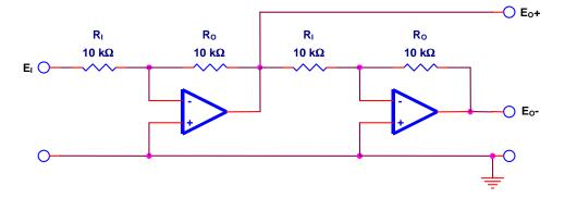
By using  $E_0$ - terminal at the reference, a p-p swing of  $4E_1$  is obtainable at  $E_0$ +, i.e. a usable swing greater than the power supply voltage rails. A fully differential operational amplifier provides this function in a single package, and is therefore the preferable design solution.
