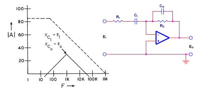
Figure 45. Differentiator With "Double Stop"
