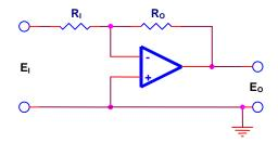
Figure 29. Equivalent Circuit of a Real Operational Amplifier
