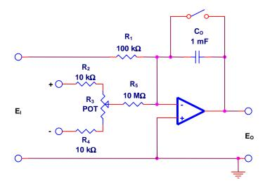
This circuit reduces current offset in operational amplifiers without "Balance" controls. With zero input and switch open, set R3 for zero output drift.
