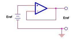
Prevent damage to standard cells induced by drawing current from them with low impedance (20 K $\Omega$  / Volt) measuring devices. See section on Buffers and Isolators for gain error. Offset adjustments should not be made with standard cell connected.
