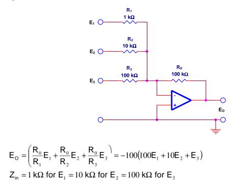
Each input is multiplied by a constant before summing-inverting output.
