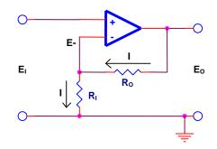
Let the voltage at the inverting input with respect to the non-inverting input be E- and the gain of the operational amplifier be A (ideally,  $A = \infty$ ).
