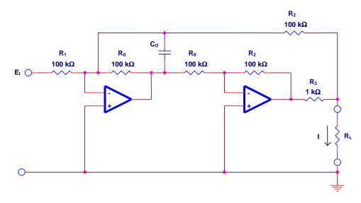
When  $R_L \ll R_2$ ,  $\frac{I_L}{E_1} = \frac{R_2}{R_1R_3} = \frac{1 \text{ mA}}{\text{Volt}}$
