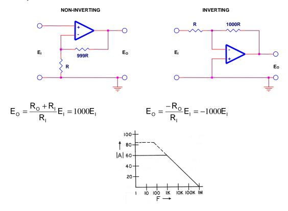
Figure 42. 60 dB Amplifier Circuits
