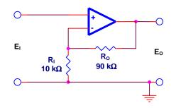
Input common mode voltage limit must be observed.
