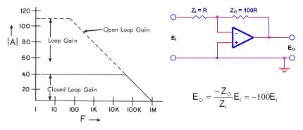
Figure 34. Closed Loop Gain of a X100 (40 dB) Inverting Amplifier
