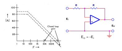
Figure 41. Voltage Inverter Circuit
