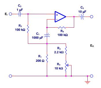
Completely developed AC amplifier with high  $Z_{in}$  and double rolloff rate and gain trim.
