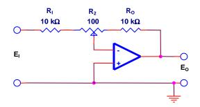
Potentiometer in feedback allows gain trimming to compensate for tolerance in resistor values.
