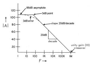
Figure 33. Sketching the Bode Plot Approximation for Figure 32
