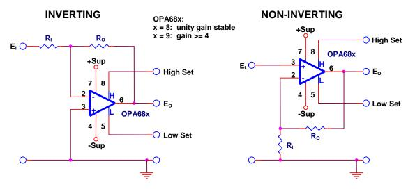
Figure 53. Voltage Limiting Operational Amplifiers
