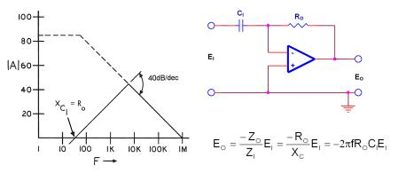
Figure 43. Differentiator Circuit
