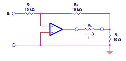
$$\frac{I}{E_1} = \frac{-R_0}{R_1R_3} = -100 \text{ mA/Volt}$$
