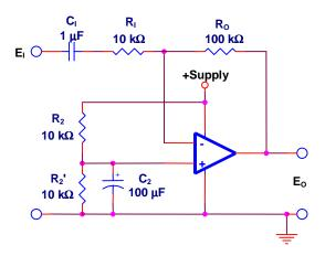
Equivalent to above, with the supply "floated" above ground.
