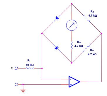
$$I_{meter} = \frac{E_1}{3R_1} = \frac{E_1}{30}mA$$
