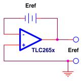
Low current drift of chopper - stabilized amplifiers improves stability and cell protection.
