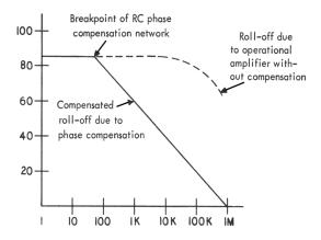
Figure 35. The Effect of Internal Phase Compensation
