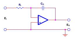
$$E_{o} = \frac{-Z_{o}}{Z_{i}}E_{i} = \frac{-E_{i}}{R_{i}C_{op}} = -\frac{1}{R_{i}C_{o}}E_{i}dt$$
