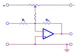
Figure 50. Inverting Amplifier with Current Offset Control
