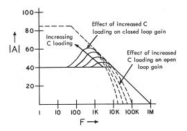
Figure 52. Gain Peaking Caused by Capacitive Loading
