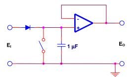
Peak value memory. Use low leakage capacitor.  $E_0 = E_1$  maximum. Common mode input voltage must be observed.
