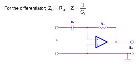
$$E_{o} = \frac{-Z_{o}}{Z_{i}}E_{i} = -R_{o}C_{ip}E_{i} = -R_{o}C_{i}\frac{dE_{i}}{dt}$$
