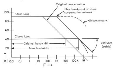
Figure 37. The Effect of Internal Compensation for Gains Greater Than 1
