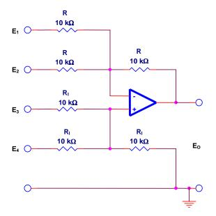
As an adder-subtracter, unused inputs should be grounded.
