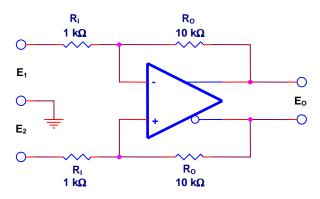
For use in driving floating loads. Input may be floating source.
