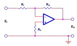
Figure 51. Drift Stabilizing the Inverting Amplifier
