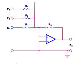
$$E_{o} = -R_{o} \left( \frac{E_{1}}{R_{1}} + \frac{E_{2}}{R_{2}} + \frac{E_{3}}{R_{3}} + \dots \right)$$
