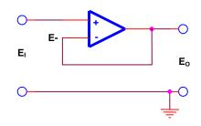
Let the voltage at the inverting input with respect to the non-inverting input be E-.
