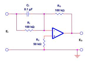
$$E_{o} = \frac{-R_{o}E_{i}}{R_{i}} - R_{o}C_{i}\frac{dE_{i}}{dt}$$
