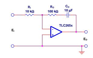
$$E_{o} = \frac{-R_{o}E_{I}}{R_{I}} - \frac{1}{C_{o}R_{I}} E_{I}dt$$
