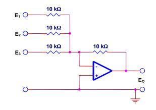
$E_{O} = -(E_{1} + E_{2} + E_{3})$  $Z_{in} = 10 \text{ k}\Omega \text{ for each input}$
